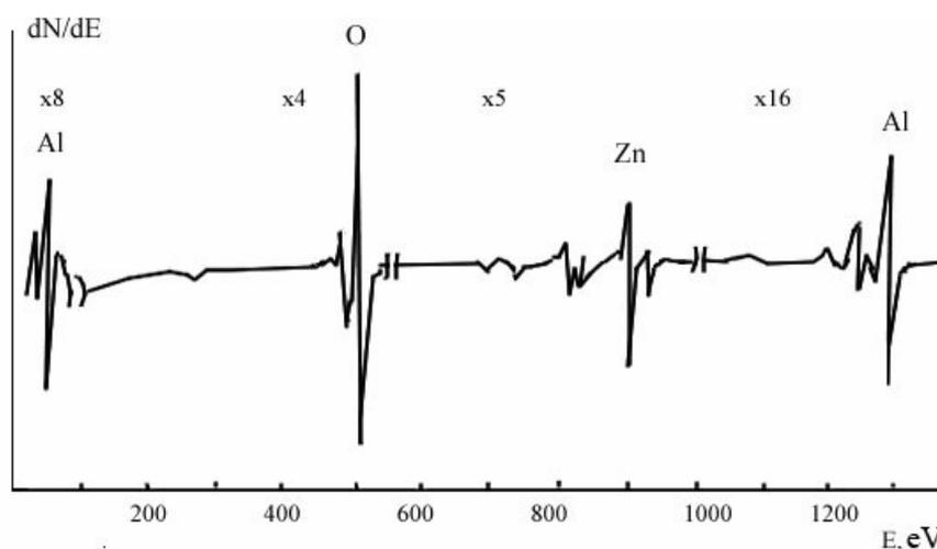
Fig. 4. Auger spectrum of the porous alumina film (the matrix) with zinc oxide nanorods grown in the pores
