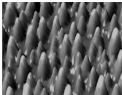
Fig. 2. SEM micrograph of ZnO nanorods
