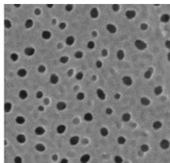
**Fig. 1.** SEM micrograph of the oxide aluminum film on the aluminum foil that was electrochemically polished under the anodizing mode with the current density  $14.0 \text{ mA/cm}^2$  (the average pore diameter is 70 nm)
