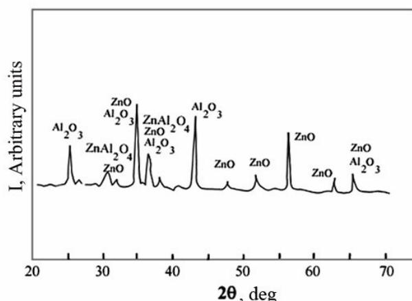
Fig. 3. A part of XRD pattern of the surface of the synthesized specimen
