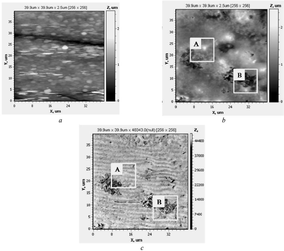
**Fig. 2.** 2D-topography (*a*) map of the surface for steel substrate of 08KP; 2D-topography (*b*) and 2D-torsion (*c*) maps of the surface for Fe-Co-Mo coating deposited in pulse mode. Scan area AFM 39.9×39.9  $\mu\text{m}$
