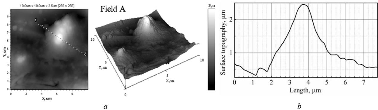
**Fig. 3.** 3D- and 2D maps of the surface (*a*) and cross section profile between markers 1 and 2 (*b*) for part A of Fe-Co-Mo coating deposited in pulse mode. Scan area AFM 10.0×10.0  $\mu\text{m}$
