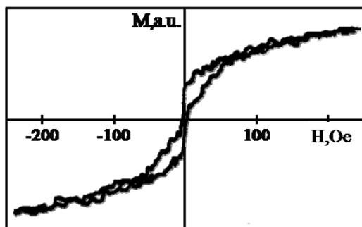
**Fig. 6.** Hysteresis loop for Fe-Co-Mo coating of composition, at.% : Fe – 47, Co – 28, Mo – 25. Substrate – copper M1
