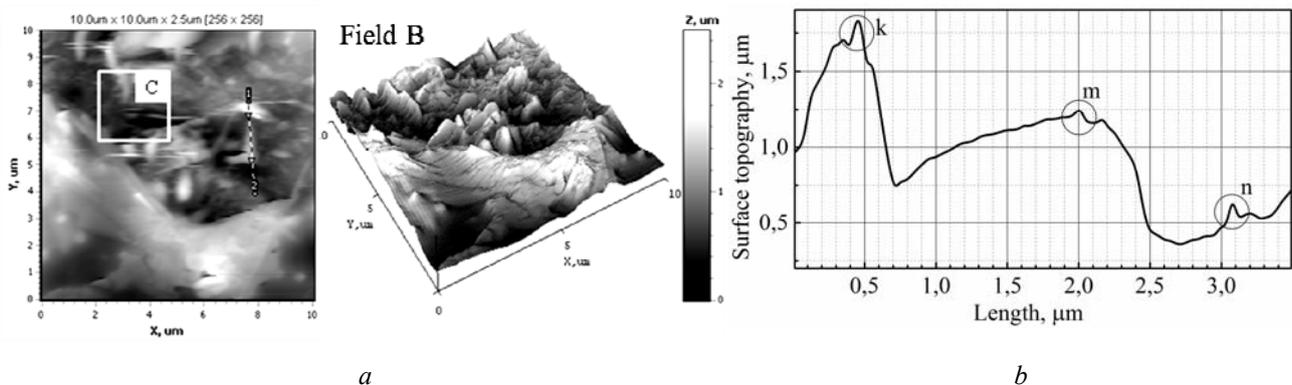
Fig. 5. 3D- and 2D maps of the surface (a) and cross section profile between markers 1 and 2 (b) for part B of Fe-Co-Mo coating deposited in pulse mode. Scan area AFM 10.0×10.0  $\mu\text{m}$
