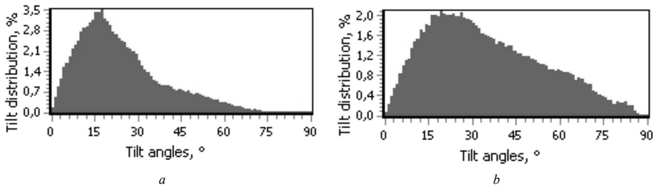
Fig. 4. Histogram of the angles to the surface normal distribution for the respective topography part A (a), part B (b)
