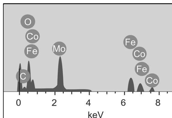
Fig. 1. EDS spectrum of the Fe-Co-Mo coating. Scan area SEM 100×100 μm
