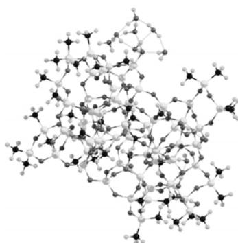
**Fig. 13.** Clustered water adsorption onto hydrophobic AM1,  $\Delta E_{1,w} = -29.0$  kJ/mol (with BSSE correction,  $\omega$ B97X-D/cc-pVDZ),  $-15.1$  kJ/mol (PM7),  $\Delta q_{1,w} = 0.033$  ( $\omega$ B97X-D/cc-pVDZ),  $0.007$  (PM7)
