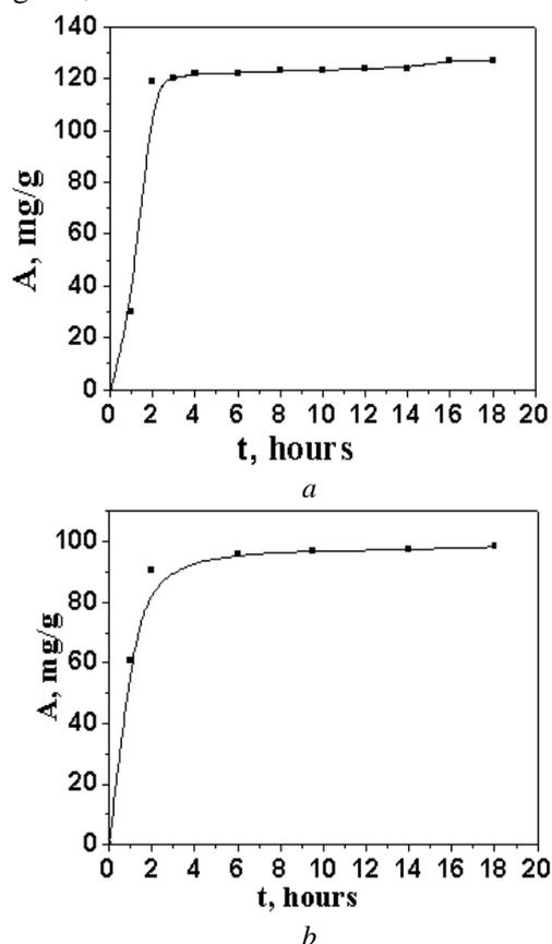
**Fig. 3.** Kinetic curves of adsorption of cisplatin at the surfaces of the magnetosensitive nanocomposites  $\text{Fe}_3\text{O}_4/\text{PAA}$  (*a*) and  $\text{Fe}_3\text{O}_4/\gamma\text{-APS}$  (*b*)
