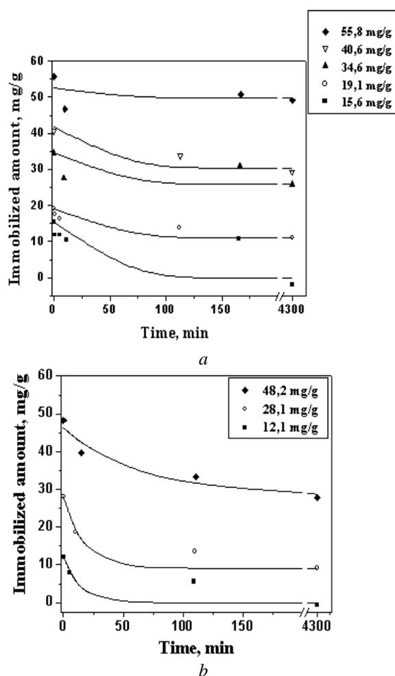
**Fig. 2.** Kinetics of release of covalently bound human immunoglobulin from the surface of the nanocomposites *a* – Fe<sub>3</sub>O<sub>4</sub>/PAA, *b* – Fe<sub>3</sub>O<sub>4</sub>/γ-APS. The initial bound amounts of immunoglobulin are shown in the right panels. The curves  $y=y(0)+Ae^{-x/t}$  were calculated from the experimental data by the method of least squares
